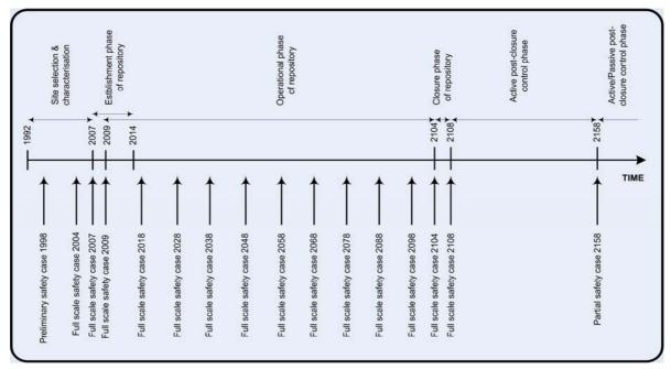
Figure 1. Safety cases within the lifetime of Bátaapáti repository
